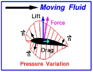
Pressure forces act normal (perpendicular) to surface. Force on the body is the vector sum of the pressure x area around the entire solid body.
