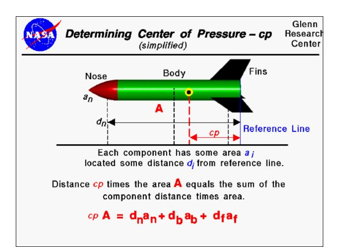
As a model rocket flies through the air, aerodynamic forces act on all parts of the rocket. In the same way that the weight of all the rocket components acts through the center of gravity (cg), the aerodynamic forces act through a single point called the **center of pressure (cp)**. How do you determine the location of the center of pressure?
