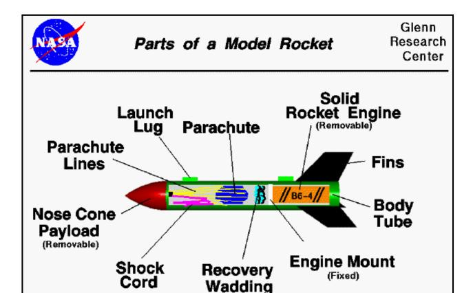
Flying model rockets is a relatively safe and inexpensive way for students to learn the basics of aerodynamic forces and the response of vehicles to external forces. Like an airplane, a model rocket is subjected to the forces of weight, thrust, and aerodynamics during its flight.
