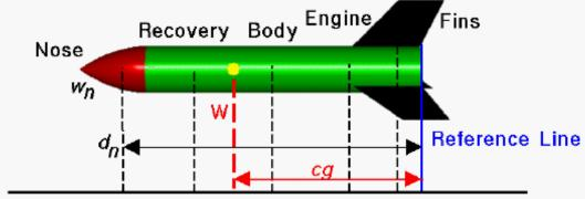
Each component has some weight  $w_i$  located some distance  $d_i$  from reference line.
