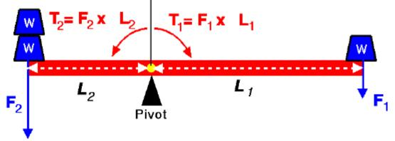
In Equilibrium (balance)  $T_1 = T_2$  $F_1 \times L_1 = F_2 \times L_2$
